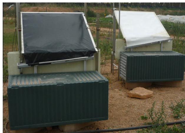
Fig. 1. View of the two radiative dew condensers with the black PE foil (BF) and the white standard foil (WSF) fitted to the 30° tilted flat pans.
